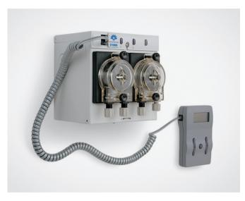
The D3000 is an extremely versatile and flexible liquid dispensing system for machine ware washing. It can dose detergent based on conductivity (probe mode), pump run time (timed mode) or speed mode (proportional) both of which are probe less.
